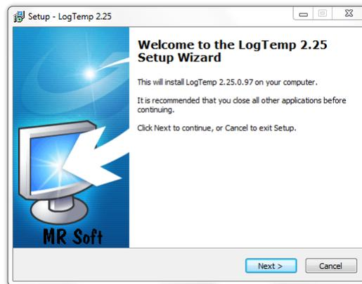
After installation start the application and in the configuration (Settings dialog) set Adapter to **COM – DS9097E** and Port COM to match your serial port name.
